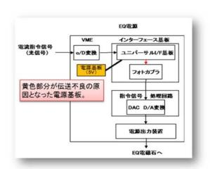
Figure 9: Flow of the control signal in the Extraction Quadrupole magnet power supply. The failure was resulted from voltage drop in a circuit board of constant voltage power supply in the yellow box.
