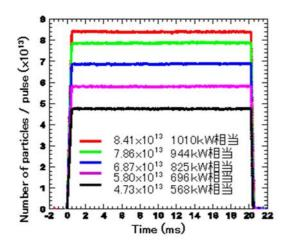
Figure 5: Beam current in the RCS from injection to extraction for various proton numbers per pulse.
