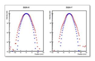
Figure 4: Beam profiles in the X and Y directions at the upstream of the SDTL section. Blue and red dots show profiles at 30 mA and 50 mA, respectively.
