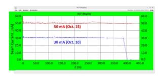
Figure 3: Beam current along the linac for 30 mA and 50 mA.
