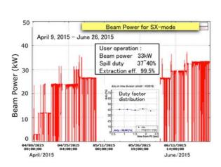
Figure 8: History of beam power at the slow extraction from the MR. Duty factor is also shown in the figure.
