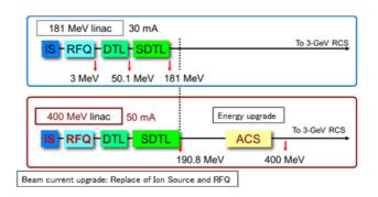
Figure 1: Schematic diagram of linac upgrade.
