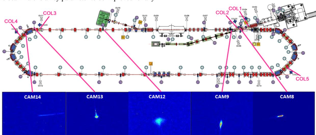
Figure 1: Layout of cERL. Collimators positions and tail profiles screen captures for laser phase +20 deg (42 ps tail).
