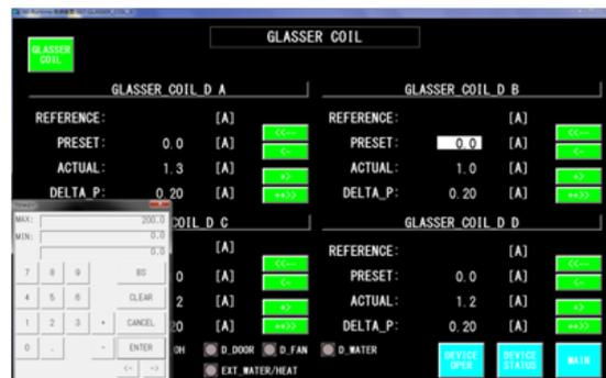
Figure 3: Photo of device control screen at the new controller.
