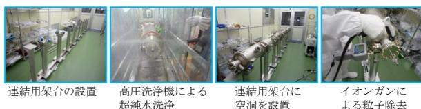
Figure 1: HPR rinsing and installation of SC cavities.
