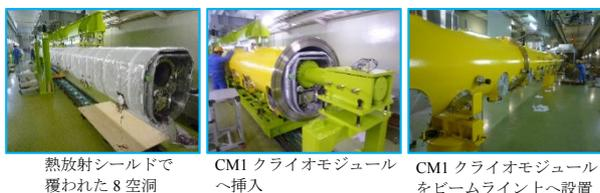
Figure 12: Insertion of cold-mass into vacuum vessel.
