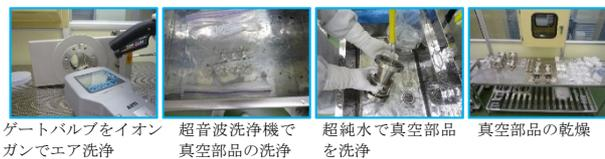
Figure 3: Rinsing of gate valves and vacuum parts.
