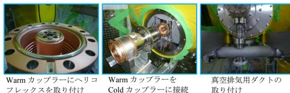
Figure 14: Installation of warm couplers.
