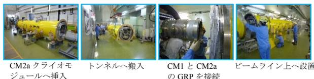
Figure 15: Installation of CM2a cryomodule in the STF tunnel.
