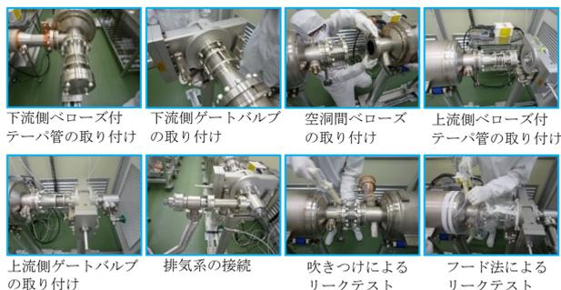
Figure 6: Assembly of gate valves and bellows.
