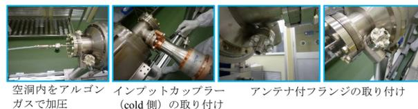
Figure 5: Assembly of input couplers and HOM coupler flanges.
