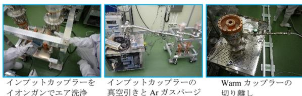
Figure 2: Cleaning and dismantling the input couplers.
