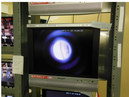
Figure 7: The ceramic window of the RF input coupler is taken by the high-sensitivity video camera. It was seen as emits light continuously.
