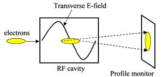
Electron bunches enters RF cavity.
