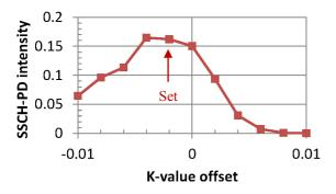
Figure 3: Bragg diffraction intensity measured by the photo-diode as a function of the K-value offset of the upstream undulators.
