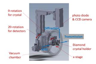
Figure 2: Diamond crystal chamber.
