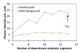
Figure 6: Peak intensity of the seeded monochromatic components and the averaged intensity of the SASE background, depending on the number of active undulator segments at the downstream of the chicane.
