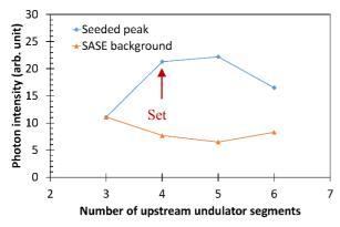
Figure 7: Peak intensity of the seeded monochromatic components and the averaged intensity of the SASE background, depending on the number of active undulator segments at the upstream of the chicane.
