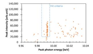
Figure 10: Distribution of the peak photon energy and the peak intensity for each single-shot spectrum, which is the same data set as "+0.05 degree" spectrum in Figure 8 d). Blue dash line box shows the criteria for "seeded" event.
