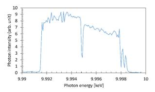
Figure 4: Energy spectrum of the transmitted SASE radiation from the upstream undulators, measured by the single-shot spectrometer with the silicon (660) configuration. There is a clear dip at 9.995 keV due to the Bragg diffraction of the diamond crystal.
