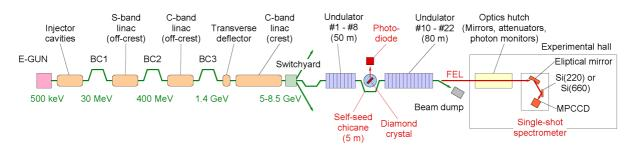
Figure 1: Configuration of the SACLA machine and the self-seeding system. BC1, BC2, and BC3 mean the three bunch compression chicanes.
