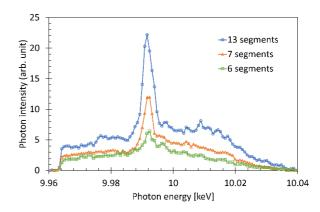
Figure 5: Energy spectra of the X-ray radiation with and without the diamond crystal, measured by the single-shot spectrometer with silicon (220) configuration. The three lines show the spectra with different number of active undulator segments at the downstream of the chicane. The spectra are the integration of 100 shots.
