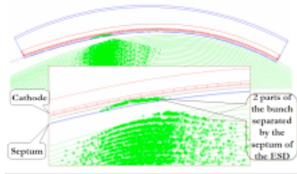
Fig 7: Simulation of the beam bunches in the extraction region.
