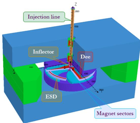
Figure 2: General view of the cyclotron computer model.
