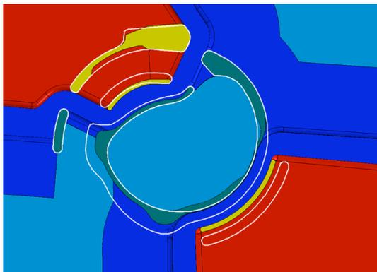
Fig 6: Renovation of the center region. White line: before renovation; yellow and green part: after renovation.
