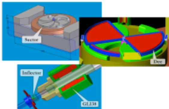
Figure 3: Some detailed parts of the cyclotron computer model.
