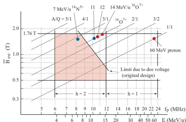
Figure 1: Acceleration performance of the AVF cyclotron. See the text for detail.
