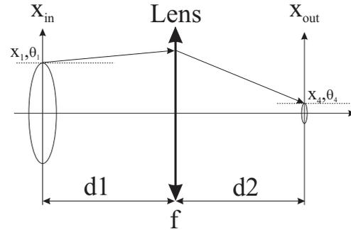
Figure 3: General geometry of one diagnostic Station of the ATF-II laser-wire LTL.
