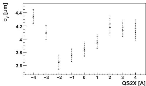
Figure 1:  $QS2X$  skew quad scan 23/05/08.  $QD4X$  set to 74 A. The grey filled circles are the Gaussian plus 0<sup>th</sup> order polynomial fits. The black triangles are the Gaussian plus 1st order polynomial fits.
