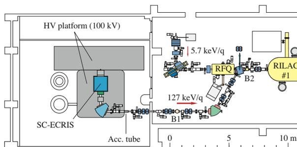
Figure 2: Configuration of the new pre-injector for the RILAC. B1 and B2 denote the bunchers operated at the fundamental frequency.
