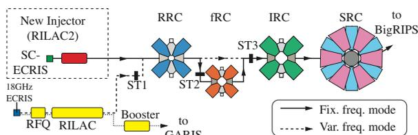
Figure 4: Expected configuration at the end of FY2010. Heavy ions such as uranium and xenon will be supplied by the new injector. Independent operation of RIBF and SHE research will be realized.
