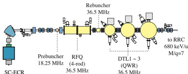
Figure 5: Schematic drawing of the new injector.
