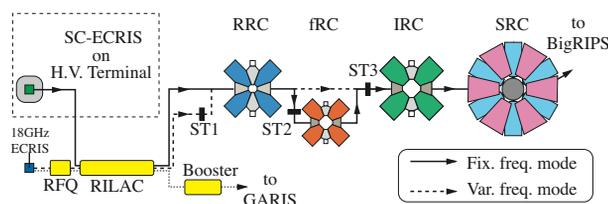
Figure 3: Expected configuration of RIBF at the middle of FY2009. Heavy ions such as uranium and xenon will be supplied from the superconducting ECR ion source on the high-voltage terminal of the Cockcroft-Walton generator.
