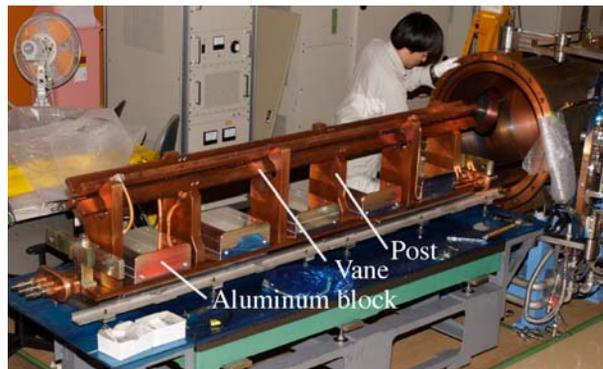
Figure 6: RFQ electrodes in preparation for the rf measurements with block tuners made of aluminum.
