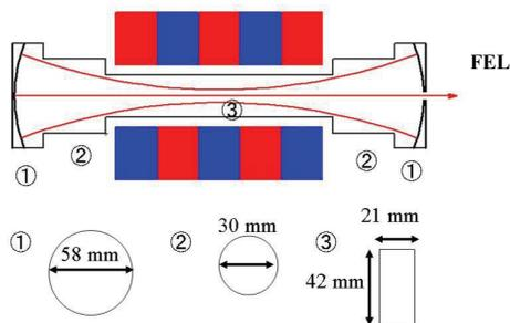
**Figure 2**, Geometry of the optical cavity of KU-FEL.
