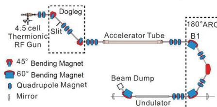
Figure 1 Schematic drawing of KU-FEL.
