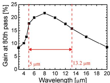
**Figure 5**, the relation between the FEL gain at 80<sup>th</sup> pass and the wavelength.
