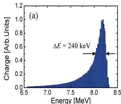
**Figure 3**, the energy spread at the exit of the RF gun.
