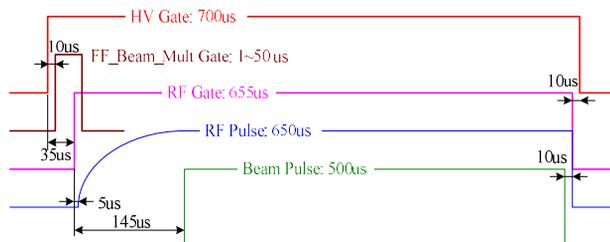
Fig. 2: Timing of the LLRF system.
