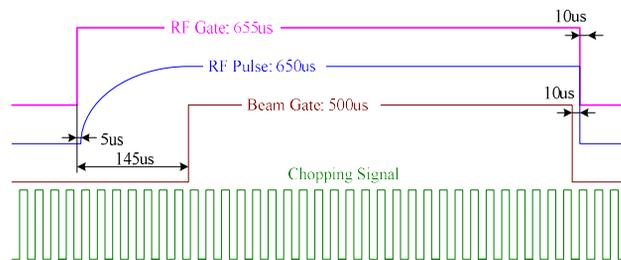
Fig. 3: Chopping signal and timing of the LLRF system.
