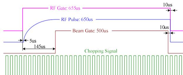
Fig. 3: Chopping signal and timing of the LLRF system.
