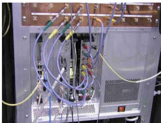
Fig. 1: Digital LLRF control system installed in a compact PCI.
