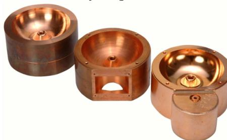
Figure 1: Linac cavity
