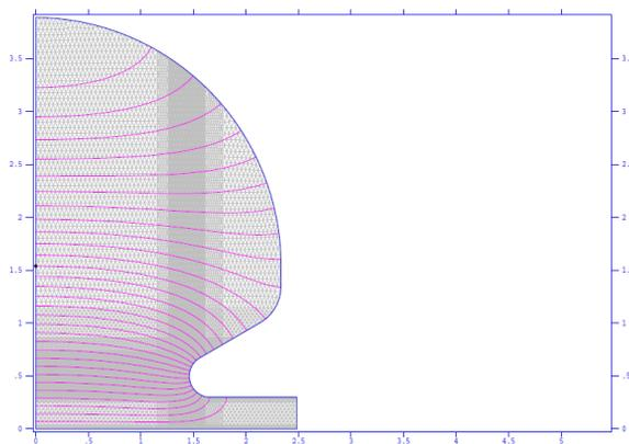
Figure 2: SuperFish plot of a single cell
