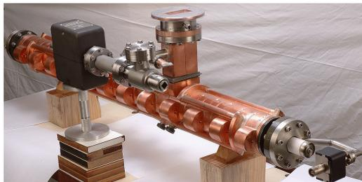
Figure 3: SAMEER made side coupled linac tube
