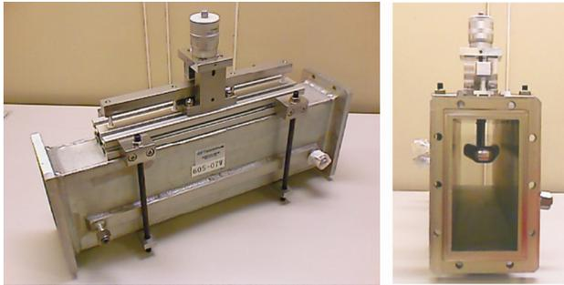
Fig. 3: L-band phase shifter based on WR650 waveguide. Phase shift  $120^\circ$ , maximum power  $> 2.9\text{MW}$ , reflection  $< -28\text{dB}$ , length 600mm.
