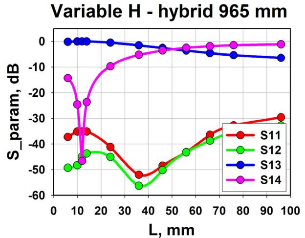
Fig. 10: S-parameters of variable hybrid with full range of coupling variation vs. fins displacement
