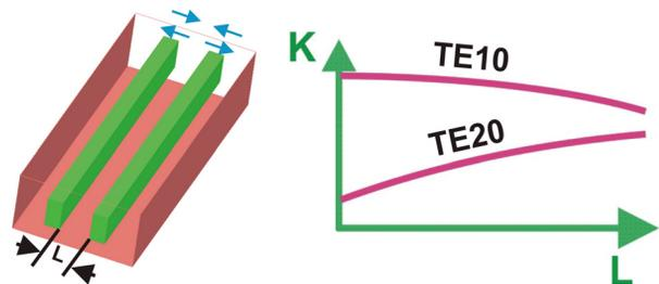
Fig. 6: Moving symmetrically and synchronically two fins in wide waveguide we can change the phase difference between modes TE<sub>10</sub> and TE<sub>20</sub>. Just exactly this property is necessary for variable hybrid
