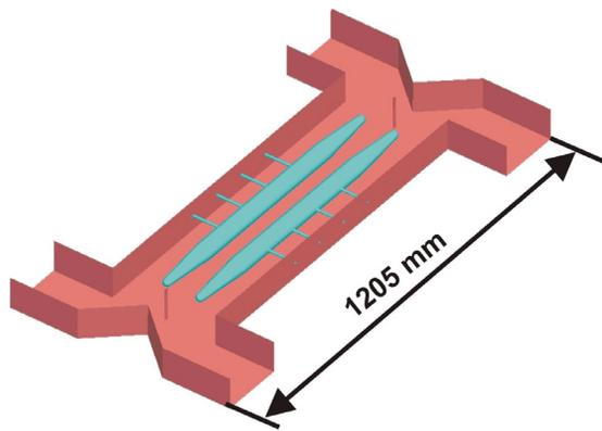
Fig. 7: Geometry of variable hybrid with full range of coupling variation. Input-output waveguides are WR650. Operating frequency is 1.3GHz
