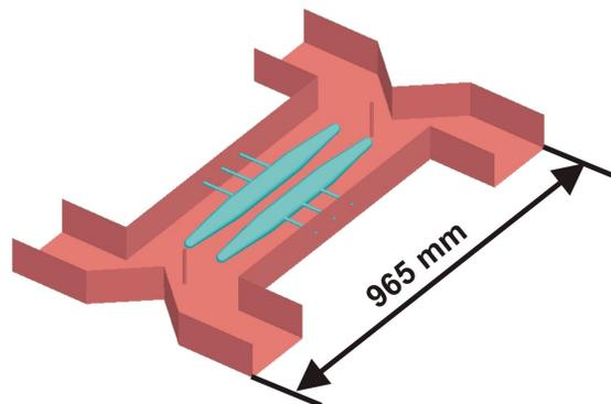
Fig. 9: Geometry of variable hybrid with partial range of coupling variation. Input-output waveguides are WR650. Operating frequency is 1.3GHz.
