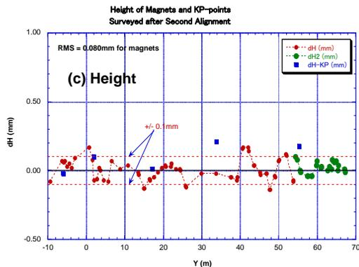
Figure 4 (c): Deviations in Z (vertical) direction. Total RMS is 0.080mm.
