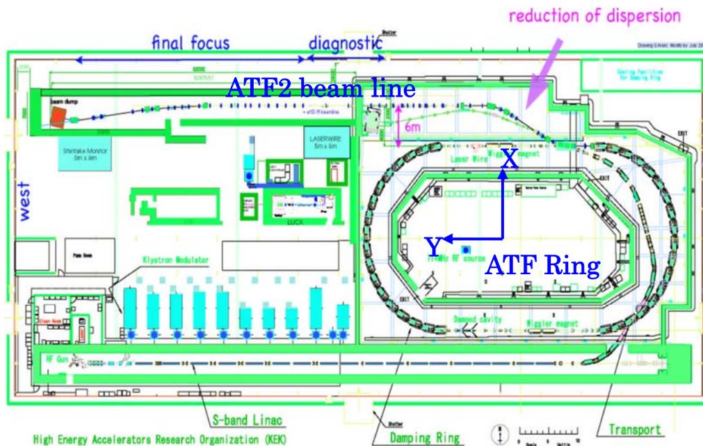
Figure 1: Layout for the ATF2 ring and the ATF2 beam line. Arrows show coordinate system.
