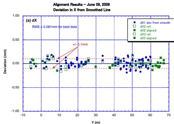
Figure 4 (a): Deviations in X direction of each magnet position from the smoothed curve. Total
