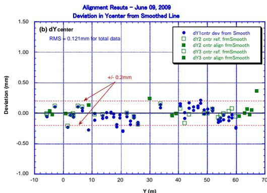
Figure 4 (b): Deviations in Y direction of each magnet position from the smoothed curve. Total RMS is 0.121mm.
