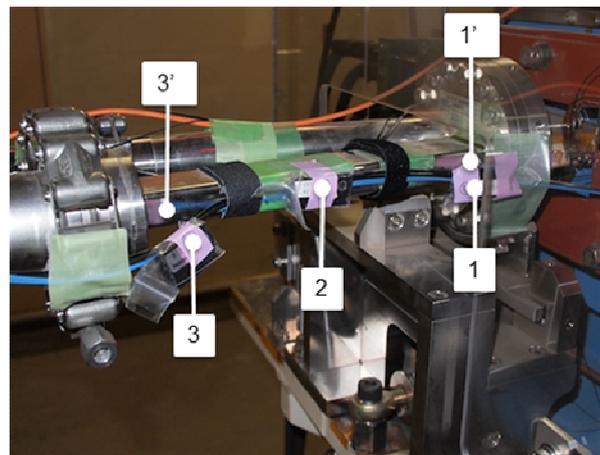
Figure 5: Photograph of optical fiber and TLD in a branch duct.
