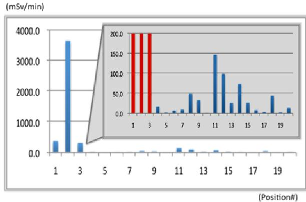
Figure 4: Dose measured by TLDs.
