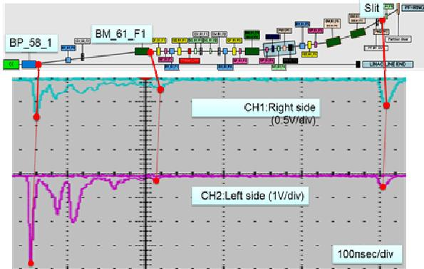
Figure 2: Oscilloscope waveform of 2 optical fibers laid on the duct in parallel, superposed with the layout of the end of the linac.
