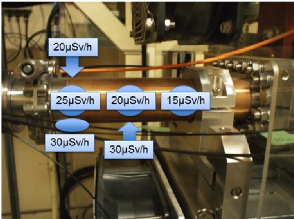
Figure 6: Measurement result on the surface of collimator of the 58\_BP\_1 upper stream.
