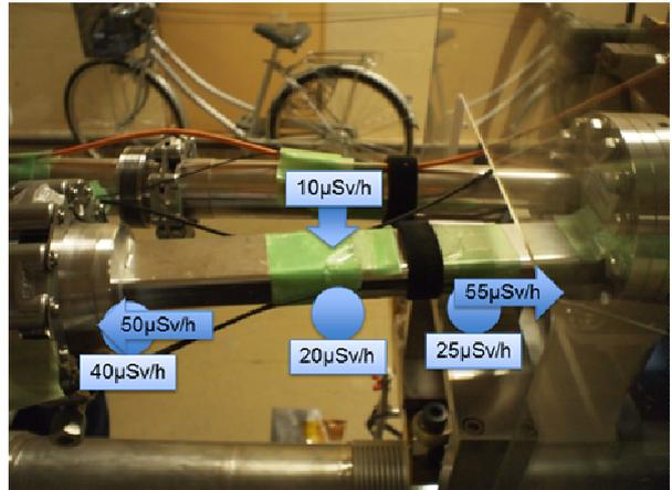
Figure 7: Measurement result on the surface of branch duct of the 58\_BP\_1 lower stream.
