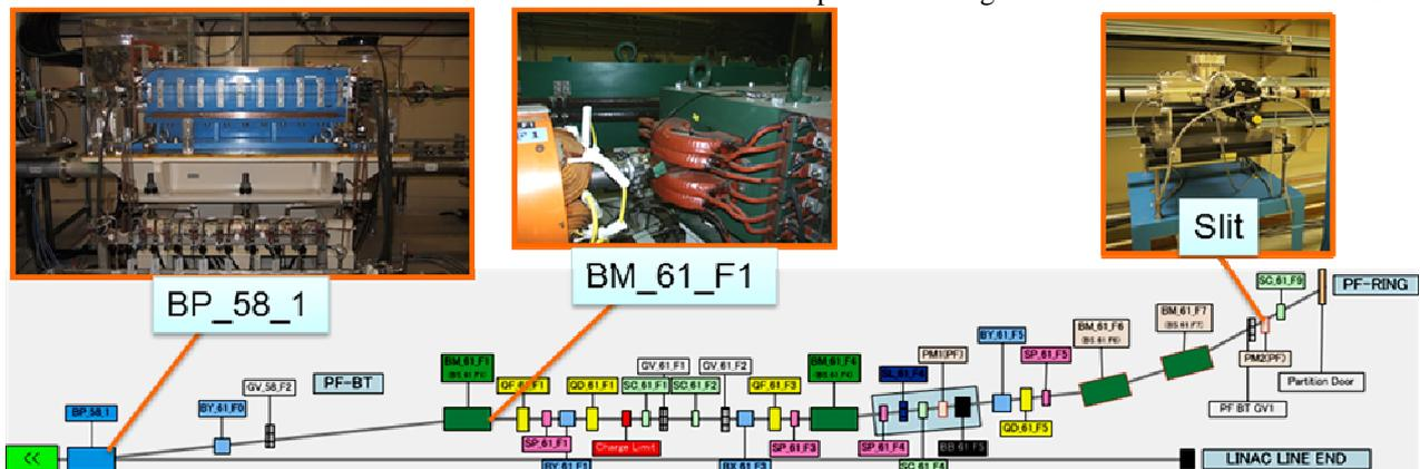
Figure 1: Layout of PF beam line in the third switching yard. The blue square represents the pulse bending magnet (BP\_58\_1); green, the bending magnet; yellow, the quadrupole magnet; light blue, the steering magnet; pink, the beam position monitor; light green, the screen monitor; red, the charge limit; and black, the beam stopper. Photographs of BP\_58\_1 and slit are also shown.
