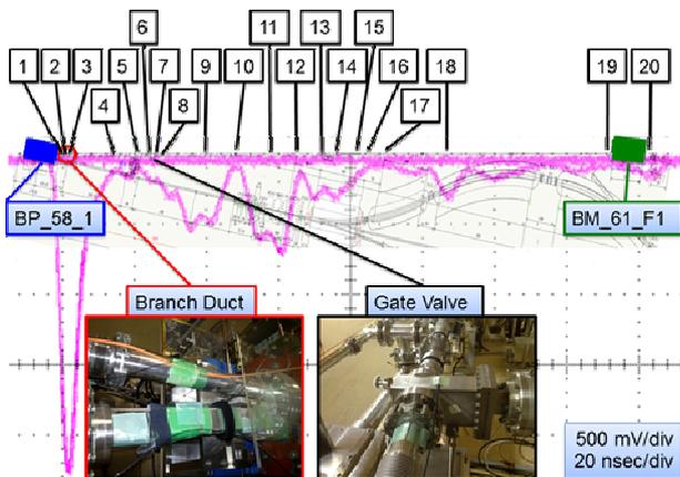
Figure 3: Setting positions of TLDs, and the signal of the optical fiber on top.
