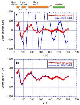
Figure 1 Measured beam response and calculated orbits. a) Orbit was calculated by original matrix, b) orbit was calculated by modified matrix.
