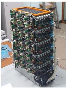
Figure 2: Solid-sate switch using SI-thyristors.
