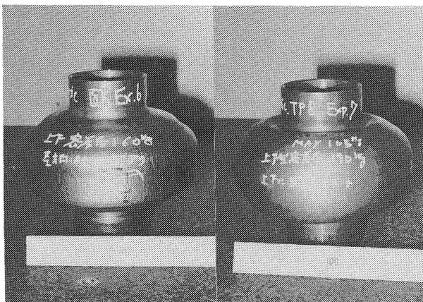
(図3). Nearly full shaped structure by hydro-bulge forming (two step included annealing).
