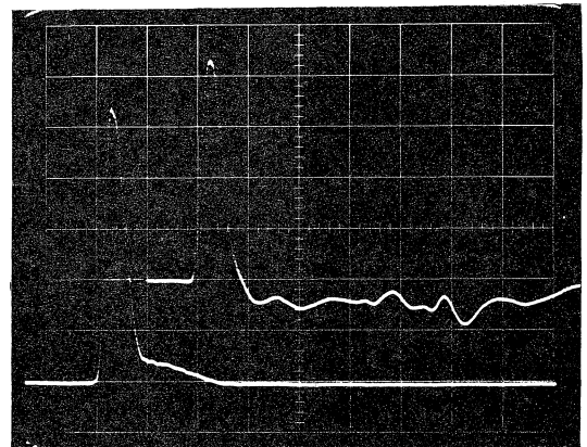
Fig.3. Input pulse(lower trace) and output pulse(upper trace) of this isolation transformer (H:5ns/div, V:20/div).
