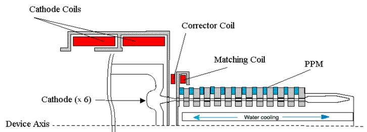
Fig 1: schematic view of the device (diode).
