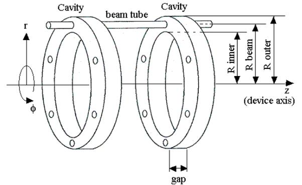
Fig 2: schematic view of the annular cavity.
