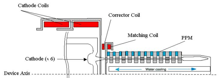
Fig 1: schematic view of the device (diode).
