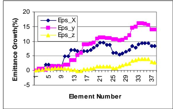
Figure 2: RMSEmittance growth along the beam line.
