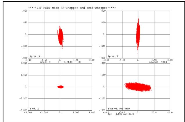
Figure 3: Phase space of a beam deflected by the chopper and the anti-chopper at entrance of the DTL.
