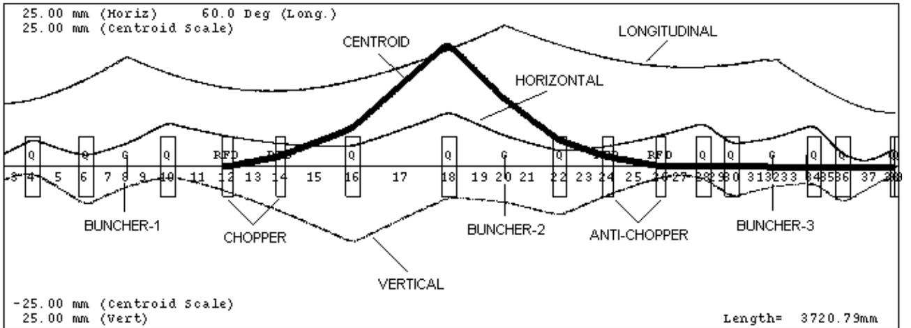
Figure 1: TRACE 3-D output of MEBT with an anti-chopper. The beam profiles in the  $z$ ,  $x$  and  $y$  directions are shown respectively. The coarse line traces the beam centroid deflected by two RF choppers and two RF anti-choppers.
