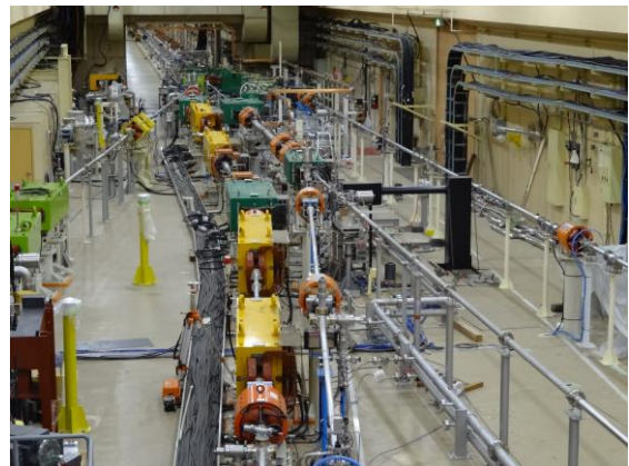
Figure 2: Photograph of the third beam switching yard at the KEK e-/e+ injector LINAC. The LINAC beam line branches to the beam transport lines with the deflecting pulsed bending magnet.
