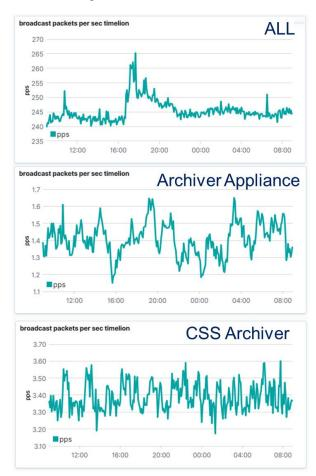
Figure 5: Broadcast packets of the KEK injector linac control network.
