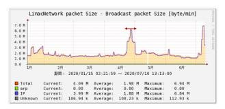
Figure 6: Broadcast packet size of the KEK injector linac control network.
