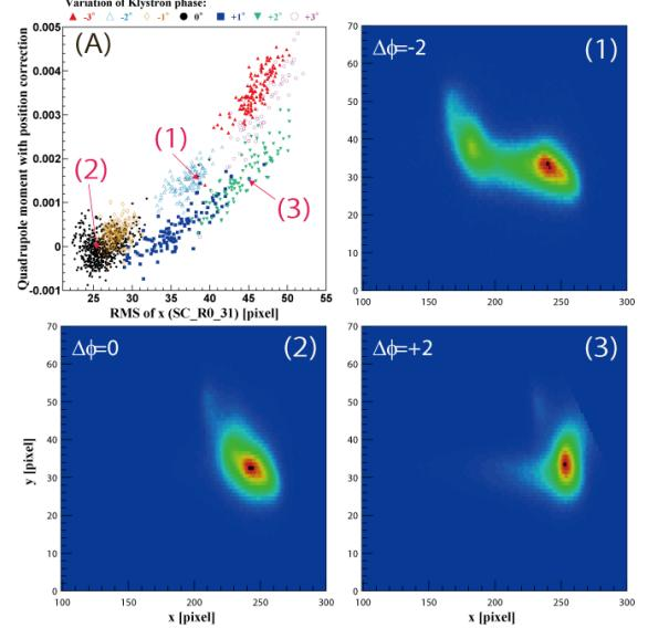
Figure 5: Quadrupole moment of the electron beam estimated by the 8-electrodes BPM and beamsize measured by the screen monitor is shown in the fig. (A). Figure (1)–(3) are beam profiles that correspond to the arrowed data points in Fig. (A).
