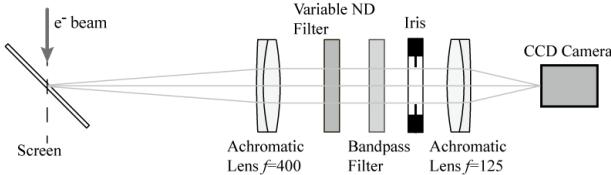
Figure 1: Layout of the optical system of the new screen monitor.
