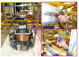
Figure 5: Pulse transformer and the broken insulator.
