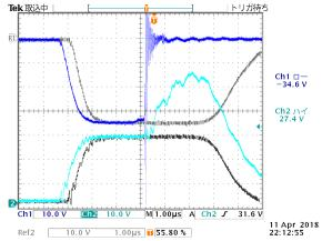
Figure 8: The waveforms when the interlock being on.
