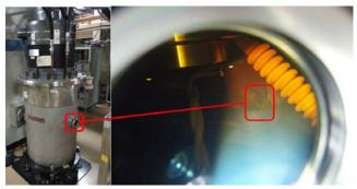
Figure 4: Broken insulator in the tank.
