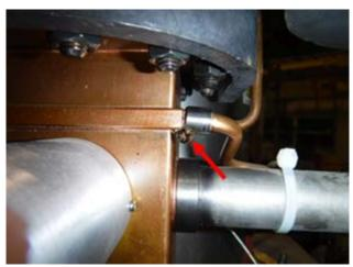
Figure 2: Water leakage at the pipe joint.
