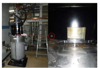
Figure 3: Water leakage from klystron magnet.
