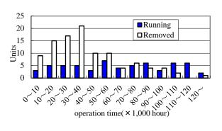
Figure 1: Klystron age profile as of March 2019.
