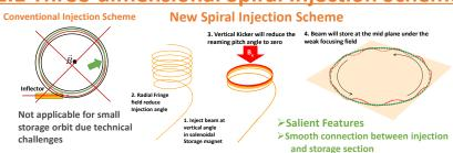
The three-dimensional spiral injection scheme is an unproven idea, therefore, a demonstration experiment to prove the feasibility of this unique scheme is inevitable. A scale down Spiral Injection Test Experiment (SITE) by the use of electron beam is under development at KEK Tsukuba campus.
