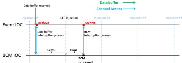
Figure 2: Time chart of data acquisition: the Event IOC receives the bunch current before injection when it receives the data buffer. That after injection is received when the BCM is processed.
