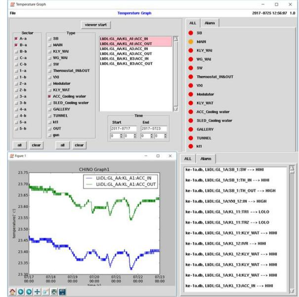
Figure 5: Image example of the new archiver data viewer and alarm display panel for managing temperature and humidity at the KEK injector linac.
