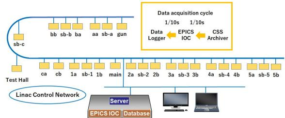
Figure 3: Schematic layout of data acquisition software for the temperature and humidity measurement system at the KEK injector linac.
