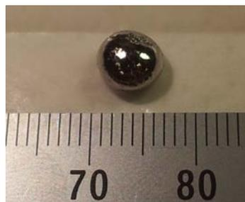
Figure 3: Photo of  $\text{Ir}_2\text{Ce}$  ingot.
