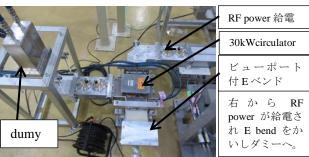
Figure 5: RF power test of 30kW circulator.
