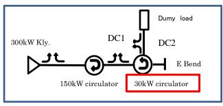
Figure 4: Test bench for 30kW circulator.
