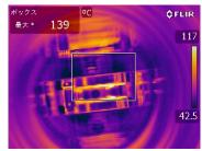
Figure 6: Inside circulator maximum temperature.
