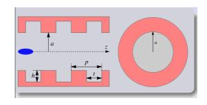
Figure 8: Schematic view of the corrugated pipe that will be used to make an energy spread of beams.
