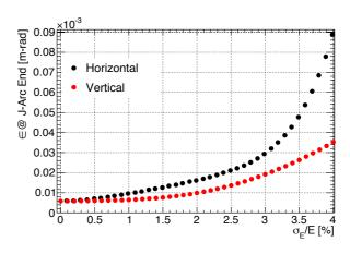
Figure 9: Emittance at the end of J-Arc as a function of an energy spread at the start of J-Arc.
