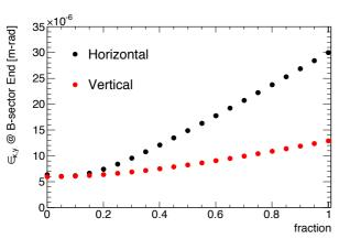
Figure 3: Emittance at the end of B-sector as a function of the fraction of the misalignment.
