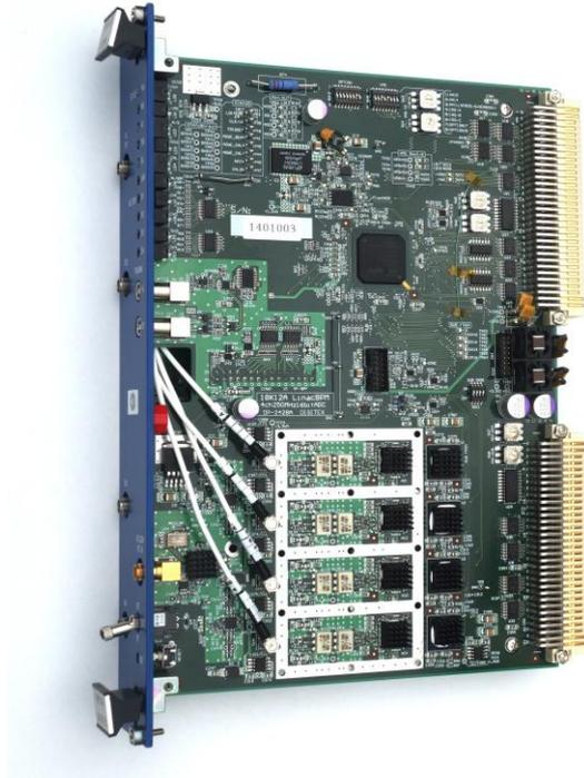
Figure 2: Photograph of prototype of BPM readout board (called 18K12A) is shown. This is double width module. BPF-Amp board is attached on bottom of the main (ADC) board. The output from BPF-Amp is fed to main board via four coaxial cables.
