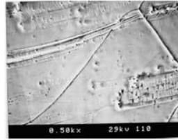
Kure furnace end copper surface mating with diamond-turned graphite
