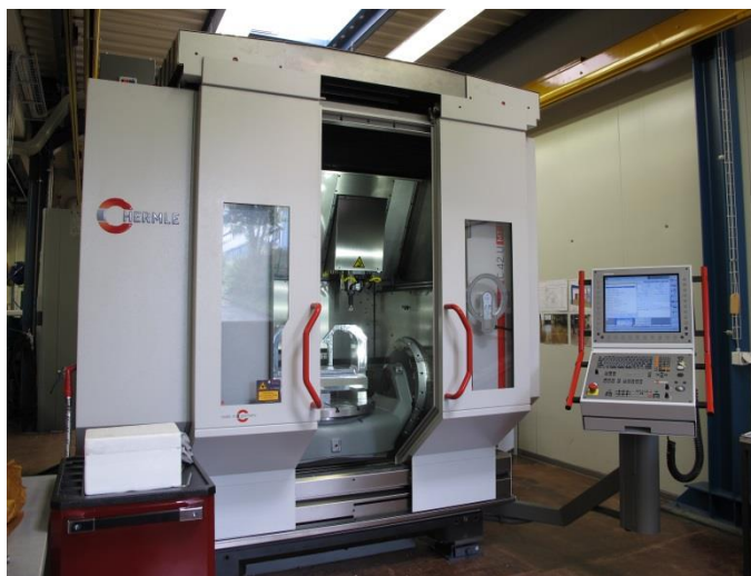
5 axes machine for BOC production (installed and operational)
