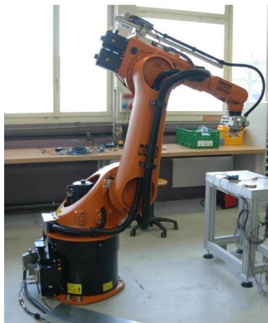
Brazing stacking provided by a robot
