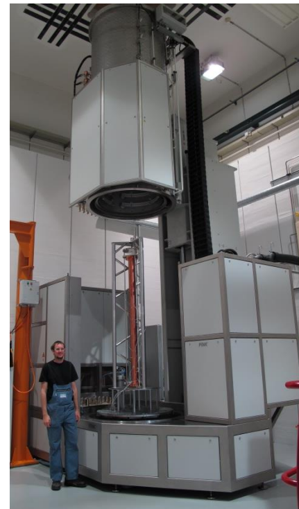
Vacuum brazing furnace installed and operative
