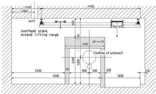
Figure 3: Cross section of Linac 1-5.
