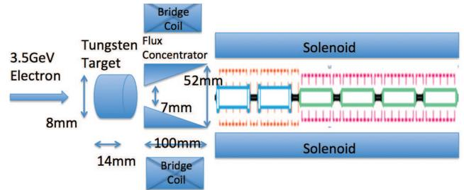
Figure 1: Schematic view of SuperKEKB positron source configuration [4].
