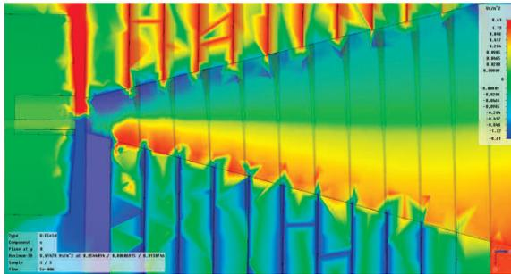
Figure 3: CST 2D FC transverse field distribution.
