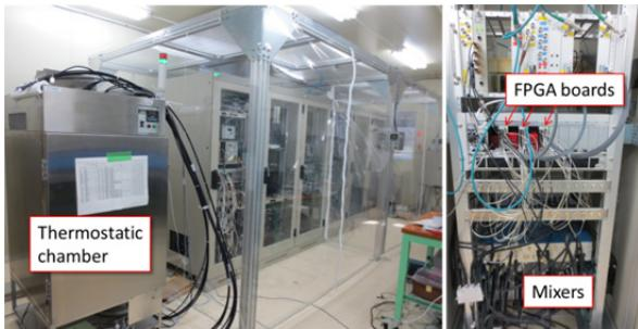
Figure 6: Photo of the LLRF control racks
