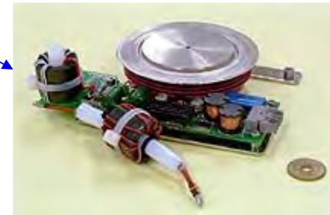
Gate driver circuit and SI-thyristor
