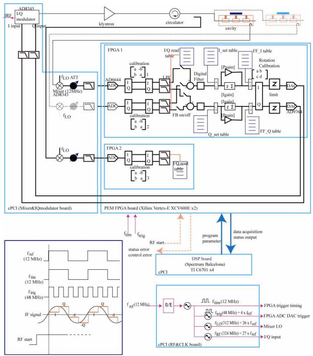
Fig. 2 FB system using FPGAs.
