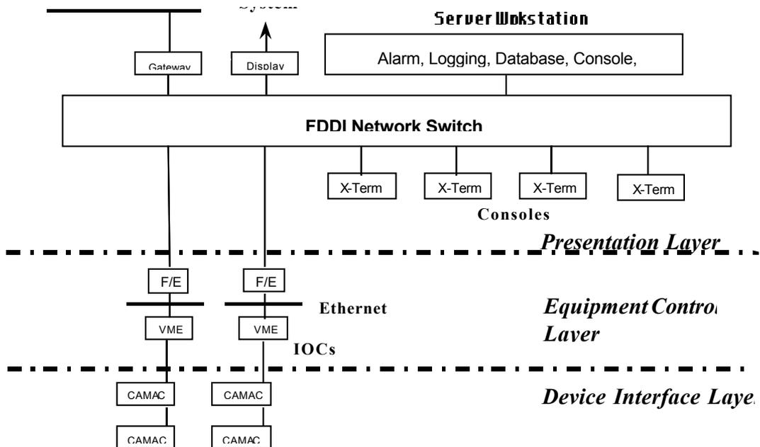
Fig. 1. System Configuration
