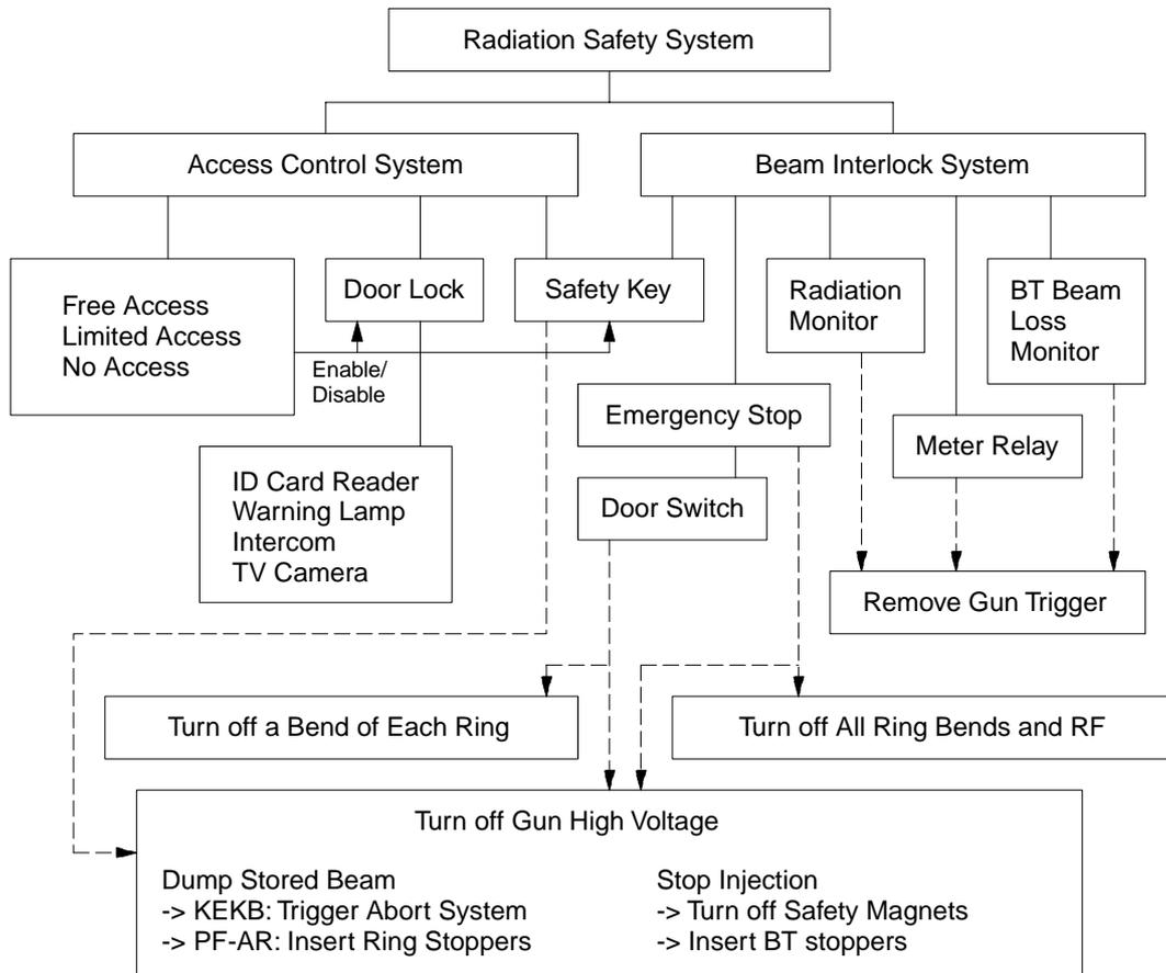
Fig. 11. Devices for access control and beam interlock.
