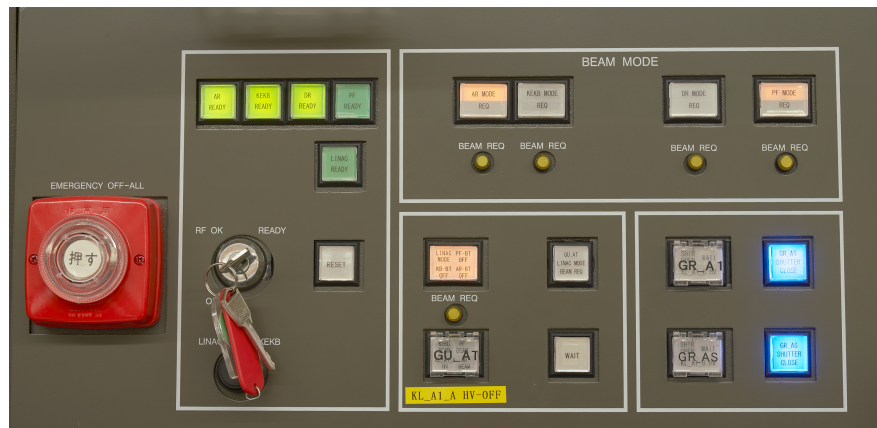
Figure 11.100: Image of the latest control panel. The beam key is used to switch the safety status from OFF, RF OK and Linac READY.
