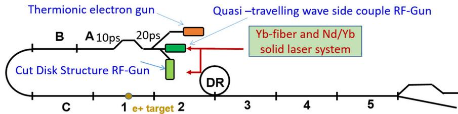
Figure 11.4: Layout of RF-gun and thermionic electron gun.
