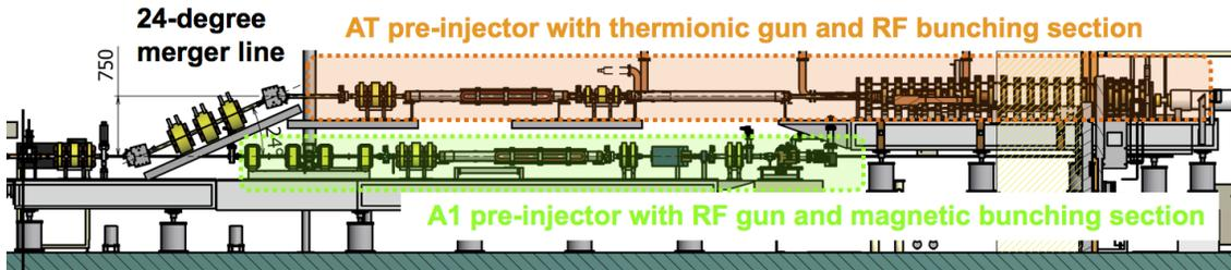
Figure 11.31: Double deck pre-injectors of SuperKEKB injector linac.
