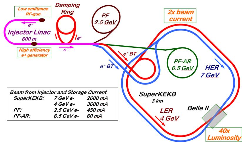
Figure 11.36: A schematic view of the electron and positron accelerator complex in the KEK.
