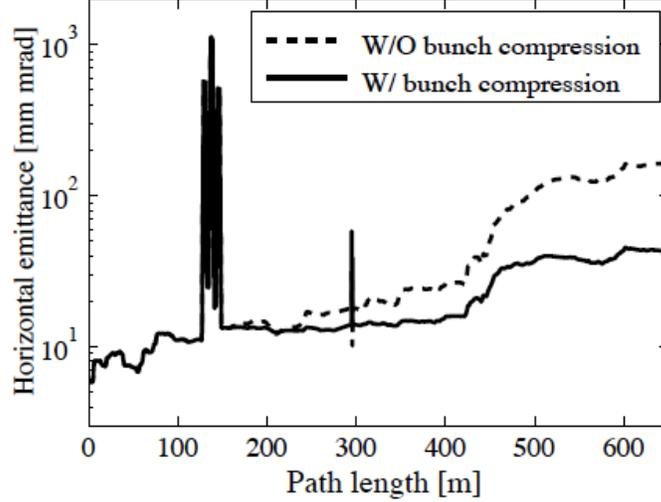
Figure 11.10: Beam tracking simulation with and without bunch compression in the J-ARC.
