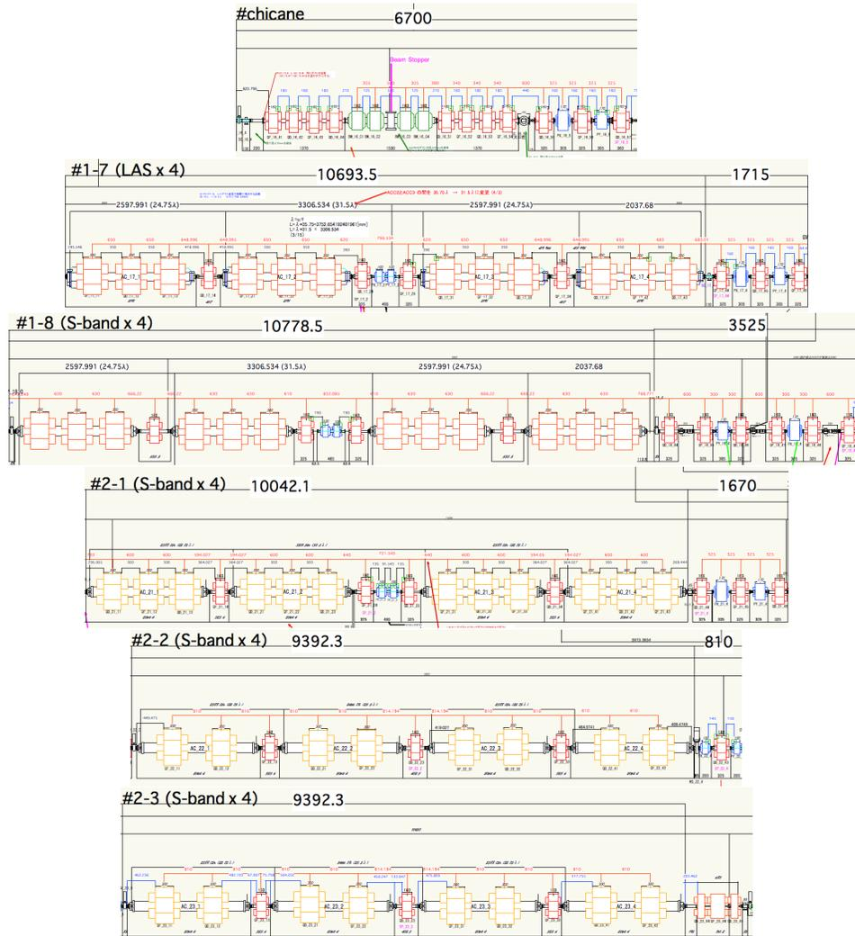
Figure 11.35: Layout of the FODO magnets in Sector-1, 2.
