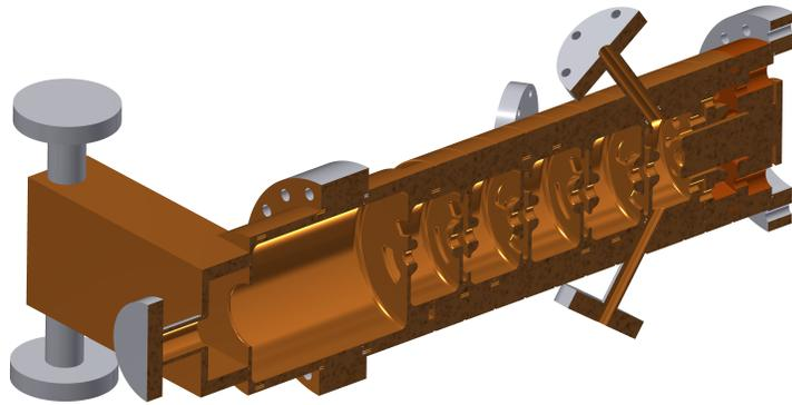
Figure 11.66: Configuration of CDS RF gun.
