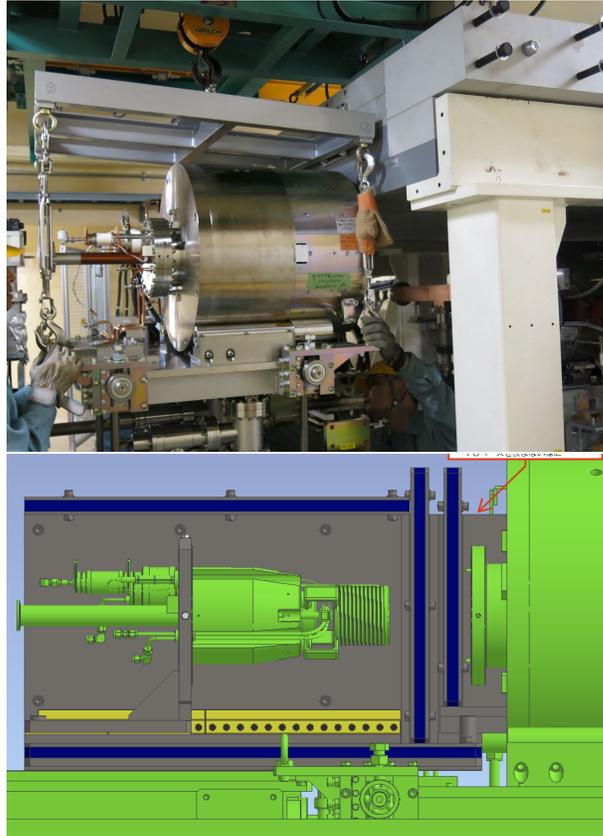
Figure 11.93: Quick exchange mechanism of FC and target
