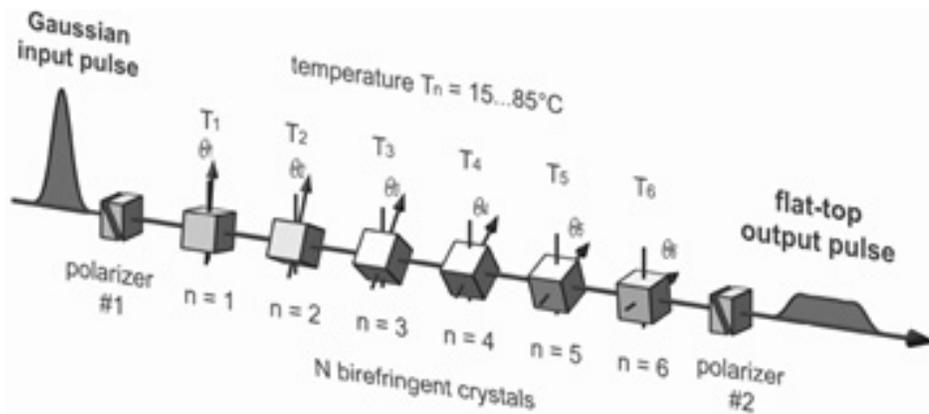
Figure 11.82: Pulse stacking technology.
