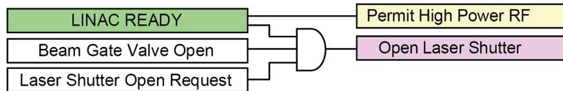
Figure 11.103: Requirements for operating the RF gun.
