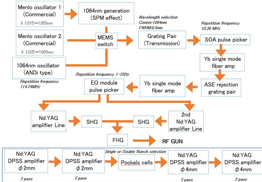
Figure 11.72: Layout of on the ground laser system.
