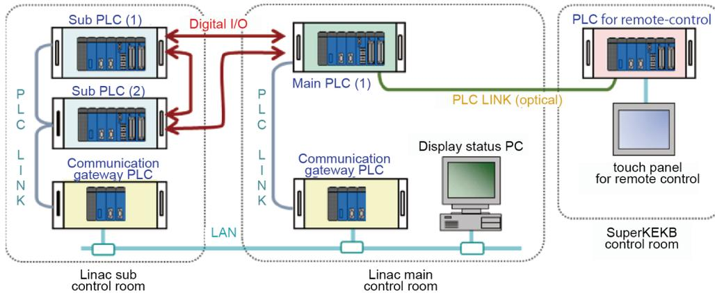
Figure 11.98: Schematic layout of the linac safety system.
