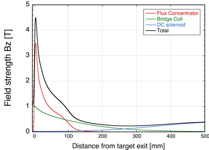
Figure 11.84: Field distribution by FC, bridge coils and DC solenoid
