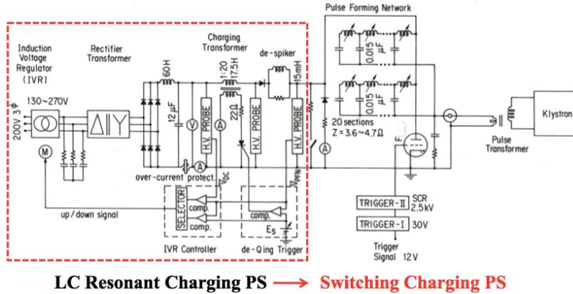
Figure 11.22: Simplified schematic diagram of the klystron modulator.
