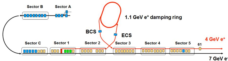
Figure 11.12: Linac schematic of acceleration unit configuration.
