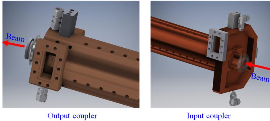
Figure 11.13: Input and output couplers of LAS.
