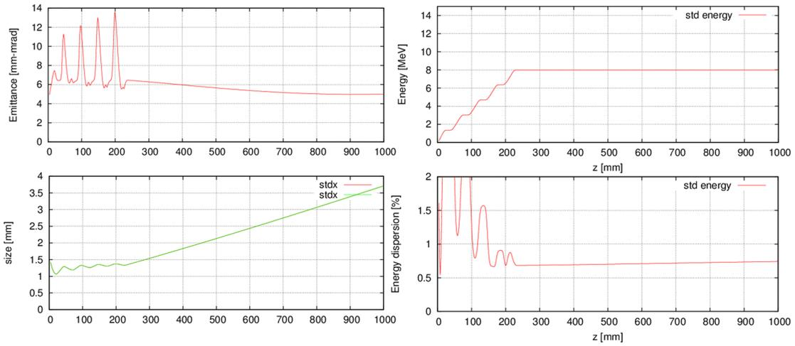
Figure 11.68: Beam tracking simulation result of emittance, beam energy, beam size and energy spread for 5 nC electron beam.
