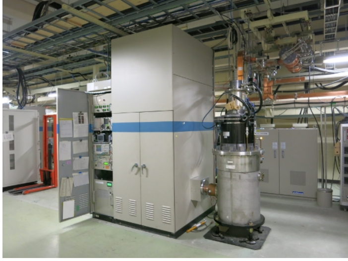
Figure 12.23: Overall view of the compact modulator with the klystron assembly and the SLED cavity.
