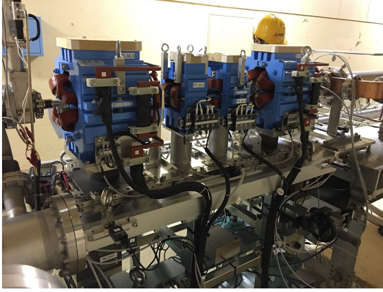
Figure 12.33: A set of pulsed quadrupole and steering magnets
