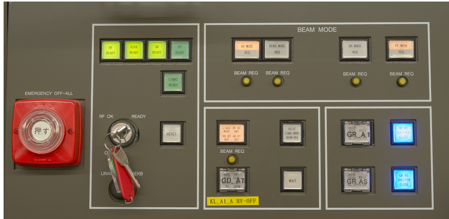
Figure 12.100: Image of the latest control panel. The beam key is used to switch the safety status from OFF, RF OK and Linac READY.
