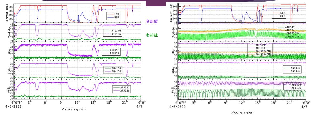
Temperature of vacuum cooling system is very stable.
