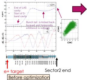
Emittance growth due to the transverse wake field of e- beam will be suppressed by the smaller beta functions with the new pulsed quads.
