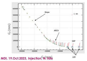
Analysis of measured electromagnet positions (2018)
