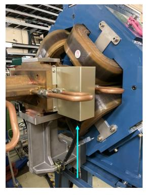
The beam pipe (BPM) is fixed to the quadrupole magnet.
