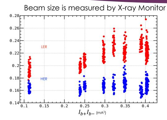
Beam size blowup is significant in LER.
