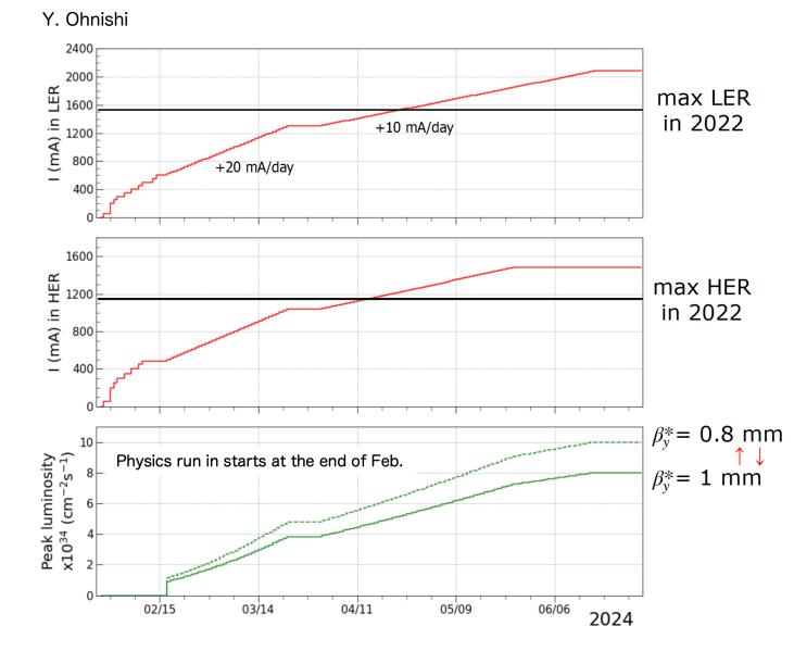
Recover the 2022 peak luminosity with  $\beta_y^* = 1mm$   $\uparrow \downarrow$   $\beta_y^* = 0.8 mm$  study  $\uparrow \downarrow$ Aim at Luminosity run with  $\beta^* = 0.8 mm$
