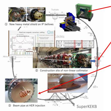
(1) Reinforcement of radiation shielding around the IP, replacement of the cap at the head of the QCS cryostat
