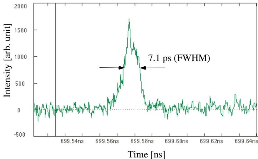
Fig. 8. Single-bunch structure of an electron beam measured by an optical transition radiation monitor at the pre-injector.
