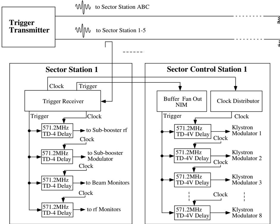
Fig. 6. Block diagram of the trigger-timing signal distribution in the sector station and the sector-control station.
