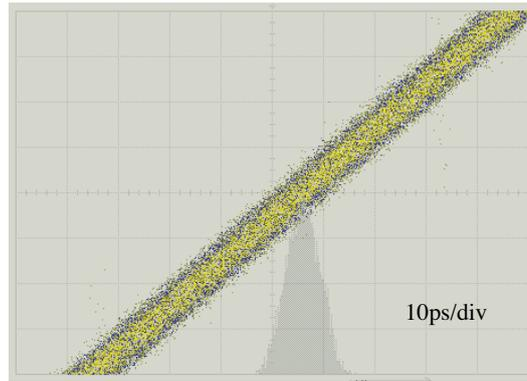
Fig. 3. Phase-jitter measurement result of the master trigger in the main station. The digital signal shows the phase jitter of the zero-cross level for the 571.2 MHz rf.
