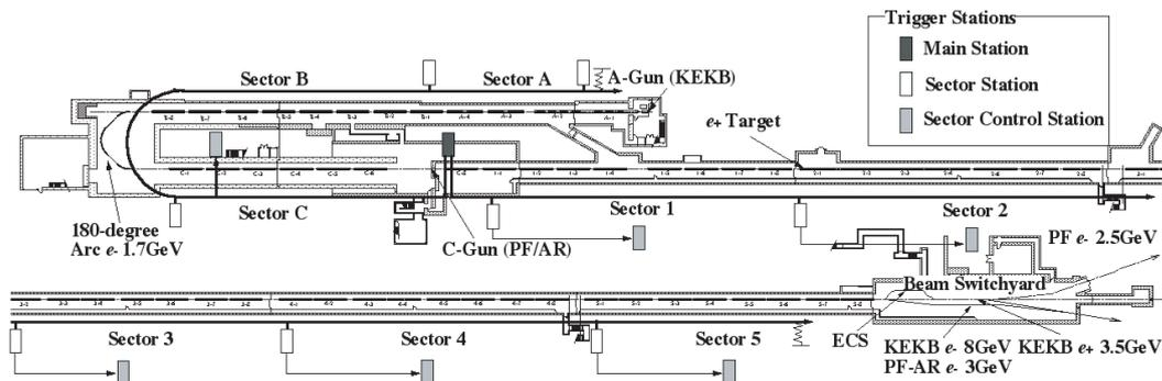
Fig. 1. Layout of the KEK electron/positron injector linac and the location of trigger stations.
