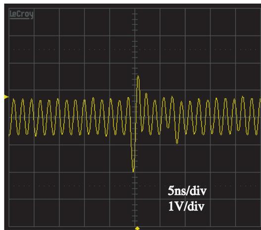
Fig. 4. Master trigger signal generated in the transmitter module.
