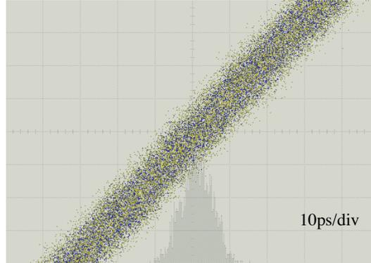
Fig. 7. Timing jitter measurement result of the trigger signal generated at sector 5. The digital signal shows the phase jitter of the zero-cross level for the 571.2-MHz rf.
