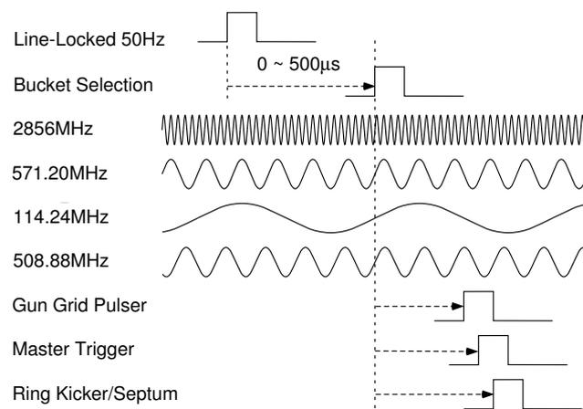
Fig. 5. Relative timing chart of the generated trigger pulses and rf signals for KEKB operation.
