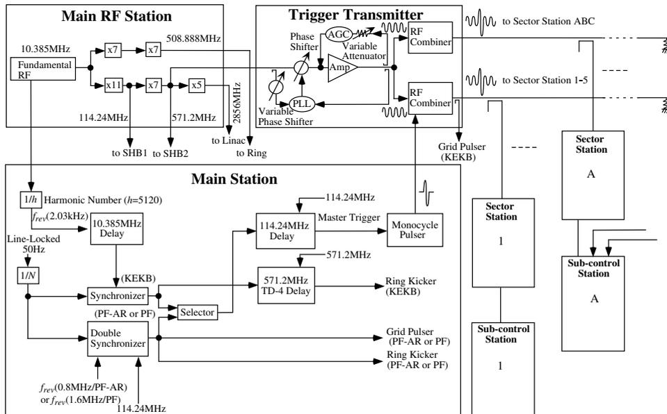
Fig. 2. Block diagram of the trigger-timing signal generation in the main station.
