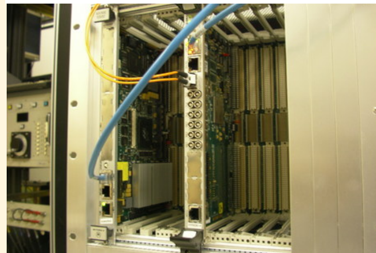
New Event Receiver Station (Timing) 16 outputs
